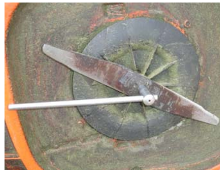
Hex socket and bar on blade nut (preferable if nut is very tight)
