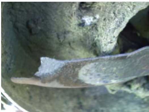
Damaged lawnmower blade
