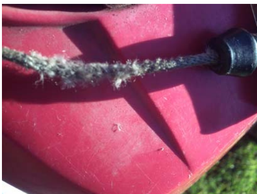
Frayed recoil starter cord
