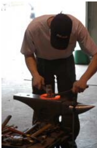
A blacksmith uses the malleability of metal to construct horse shoes
